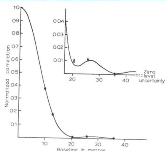
Fig. 11.5. Correlation as a function of baseline for Sirius A ( $\alpha$  C Ma). The points show the observed results; the full line shows the theoretical curve for a model atmosphere ( $T_e = 10,000$  K,  $\log g = 4$ ,  $\lambda = 450$  nm). Results for three long baselines are shown on an expanded scale together with their r.m.s. uncertainties. (Total exposure 203 hours.)
