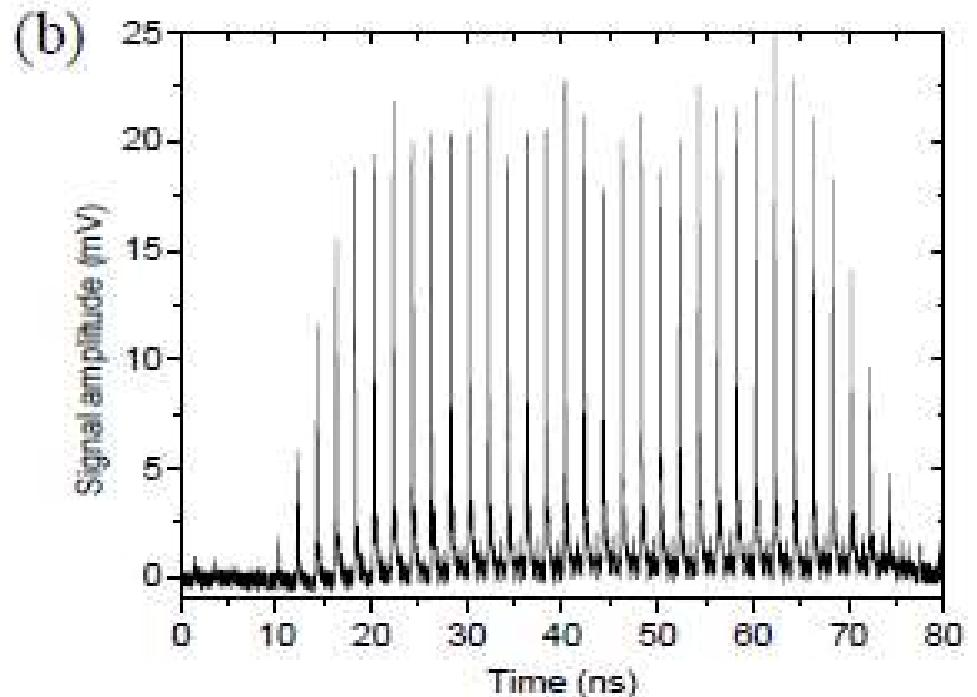
Fig. 3 (a) Measured detector signal of a 15 nm YBCO THz HEB over time. The distance between two trains is 20 ns (50 MHz). In (b) one train with 33 bunches is depicted in detail.
