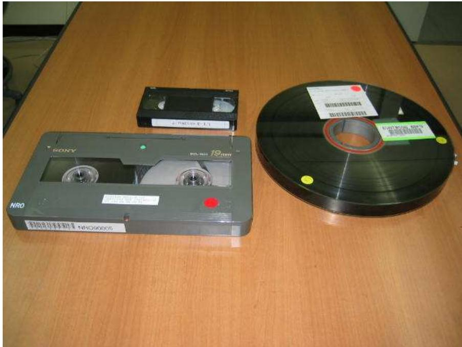
Figure 42: Magnetic tapes used in VLBI: S2 (top left), K-4 (left), and VLBA/Mark IV (right).
