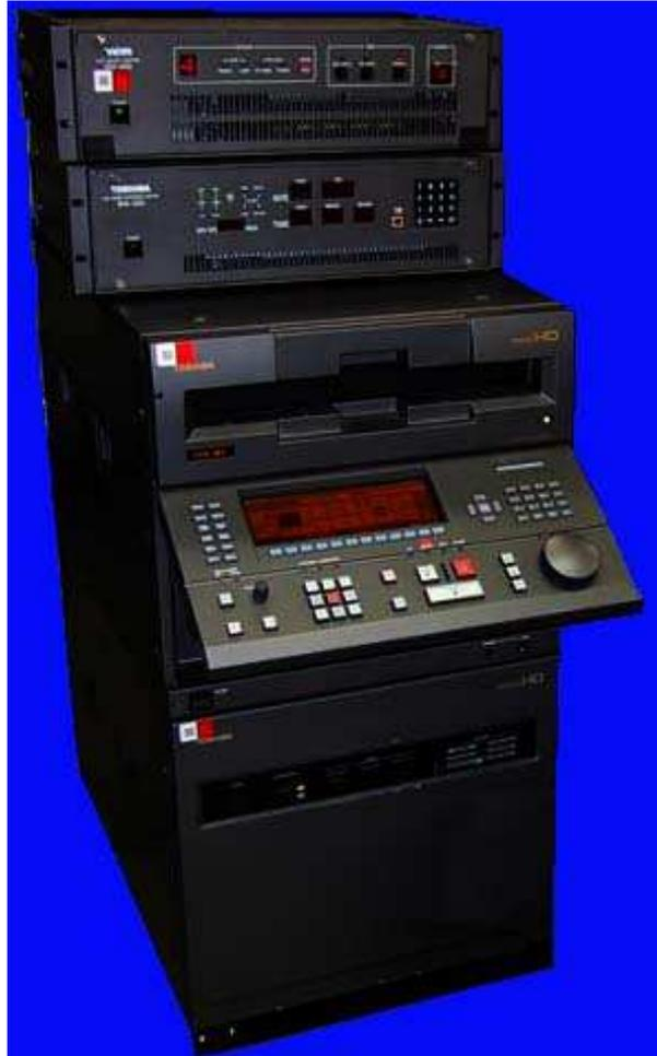
Figure 52: GBR-1000 1 Gbps VLBI system based on an HDTV video cassette recorder.
