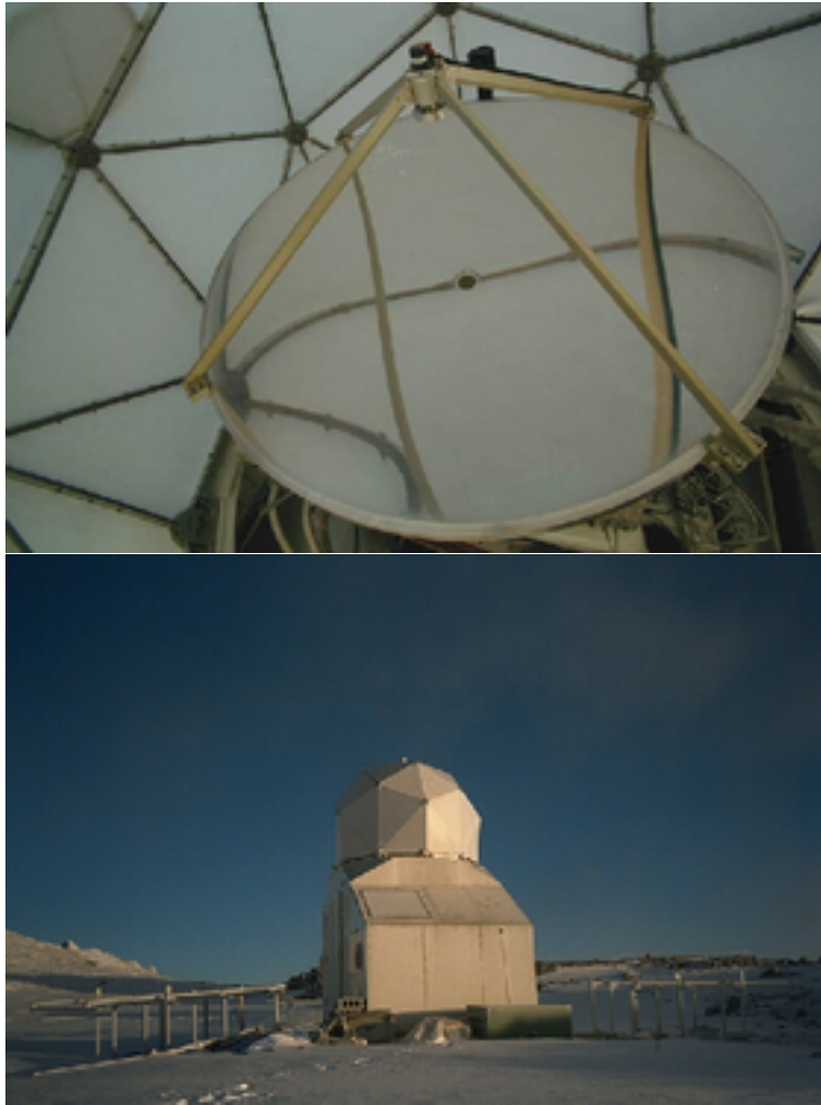
Figure 12: Main reflector (top) and radome (bottom) of the 1.2 m submm-wave telescope at the top of Mount Fuji, Japan.
