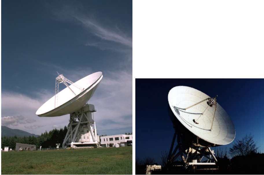
Figure 8: A flexible 45 m Millimeter–Wave Telescope at Nobeyama, Japan (left), and a “stiff” 32 m geodetic VLBI antenna at Tsukuba, Japan (right).
